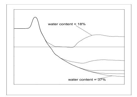
FIGURE 7-3. Waveforms collected in a sandy loam using CS610 probe with RG8 connecting cable. Volumetric water content values are 10, 18, 26, 30 and 37%. Solution electrical conductivity is 10.2 dS m<sup>-1</sup>.
