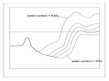
FIGURE 7-2. Waveforms collected in a sandy loam using CS610 probe with RG8 connecting cable. Volumetric water content values are 10, 16,18, 21 and 25%. Solution electrical conductivity is 1.0 dS m<sup>-1</sup>.
