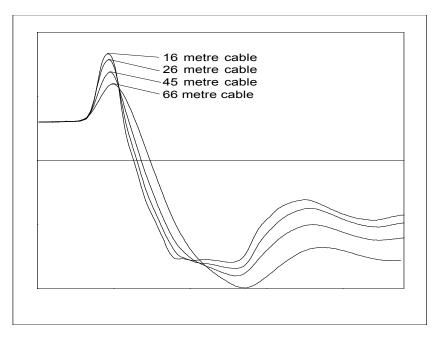
FIGURE 7-1. Waveforms collected in a sandy loam using CS610 probe with RG8 connecting cable. Volumetric water content is 24% and bulk electrical conductivity is 0.3 dS m<sup>-1</sup>.
